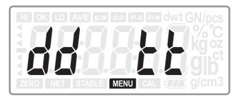
Press **ENTER** key to display the date mode for setting (flickering for 3 seconds)
