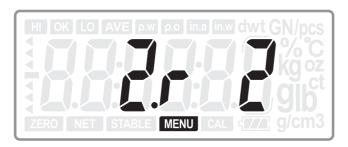
Press T or A key to select the range of zero return range from 0 to 3. (The larger the number selected, the shorter time for zero return) (Default: 2)
