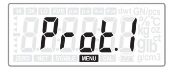
Press or A key to choose the available protocols: Prot1 (MWP), Prot2 (22byte) or Prot3 (MW-II)
