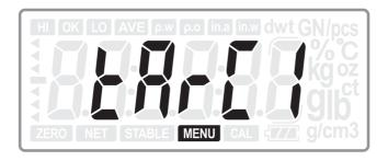
Press **ENTER** key to confirm the choice and return to normal weighing mode; or press  $\frac{\text{SAMPLE}}{\text{Back}}$  **Back** key to return to last step
