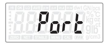
Press **ENTER** key to enter into the serial port setting:
