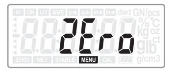
Press ► T or A key to select the IR key function: ZERO, TARE, PRINT or Off. (Default: ZERO)
