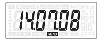
Press  $^{\bullet}$ T $^{\triangleleft}$  or  $^{\bullet}$  key to increase or decrease the number (yy:01-99; MM: 01-12; dd: 01-31); press  $^{\bullet}$ O $^{\triangleleft}$  key to move the digit.
