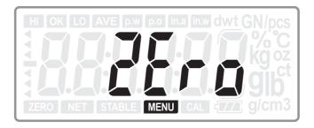
Press To or A key to select the IR key function: ZERO, TARE, PRINT or Off. (Default: ZERO)
