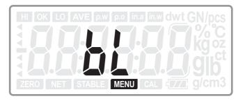
Press **ENTER** key to enter into backlight mode setting:
