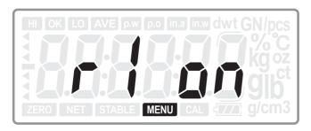
Press T or A key to choose the serial ports: R1, R2 or USB; press 0 key to choose the ports to be on or off. (R1-RS232C1 for CD-300 remote display; R2-RS232C2 for PC and printer)
