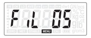
Press To a key to select the range of stability from 1 to 15. (The larger the number selected, the shorter time for stable state) (Default: 05)
