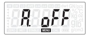
Press **ENTER** key to enter into the shut off time setting:
