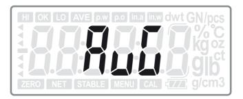
The AVG character flickers for 2 seconds and then it displays the weight. (The weight is an average weight value)
