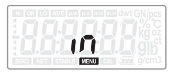
Press To r A key to set the alarm type: IN or OUT. (Default: OUT)
