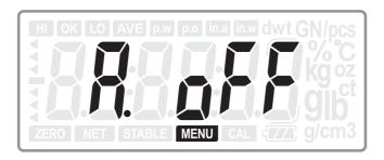
Press **ENTER** key to enter into the shut off time setting:
