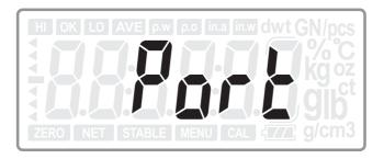
Press **ENTER** key to enter into the serial port setting:
