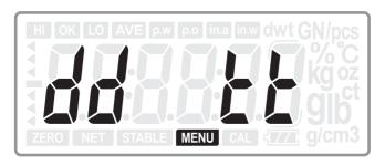
Press **ENTER** key to display the date mode for setting (flickering for 3 seconds)
