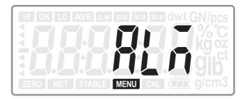
Press **ENTER** key to enter into alarm mode setting:
