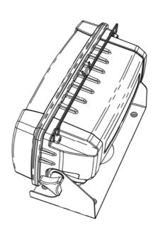
Attachment of Lead Seal through optional Captive Security Screws. Please note that security screws are available as an option and that they are less corrosion resistant than the standard Captive Screws.
